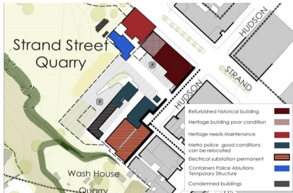
Figure 2.21: Condition of buildings in the study area (Meyer and Associates, 2023)
